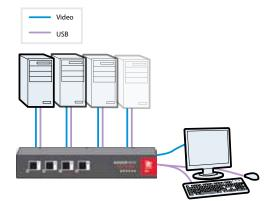
The switching section is hard wired to allow only one channel to be selected at any time.
